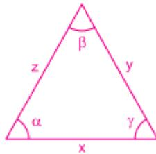
$$1.^{\circ}) \frac{y}{\text{sen } \alpha} = \frac{z}{\text{sen } \gamma} \Leftrightarrow \frac{\text{sen } \alpha}{\text{sen } \gamma} = \frac{y}{z} = 1 \Leftrightarrow y = z$$
